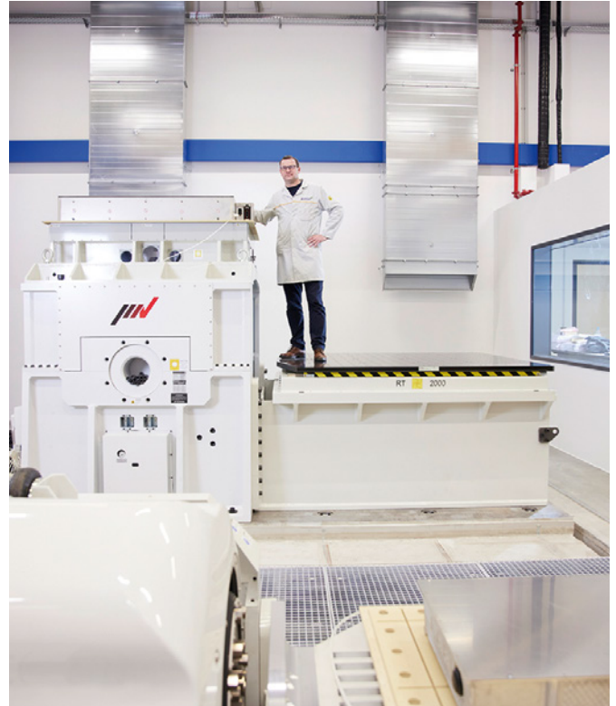
Endurance test for battery systems: The 16 tons shaker is used to simulate loads from real-world operation
