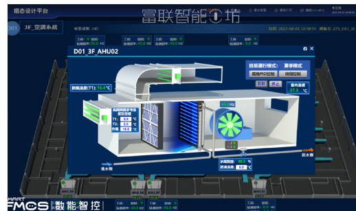
Operation Screen of Air-conditioning System
