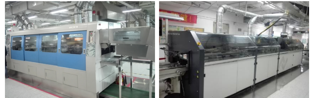
Application of Wave Soldering Technique (Left: Outdated Equipment; Right: New Energy-saving Equipment)
