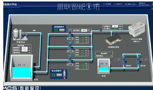
Monitoring Screen of Water Pump Room
