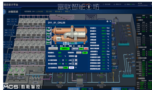
Operation Screen of Water Chiller
