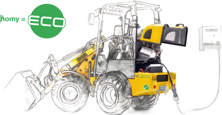
WL20e: first zero-emissions wheel loader.
