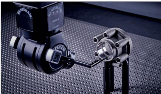
Our products enable customers to maximise the potential of their capital equipment; the REVO-2 measuring system for CMMs allows a range of inspection applications on a single machine, including dimensional and surface finish measurement.
