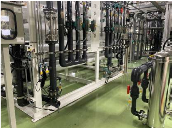
By filtering and treating wastewater from cutting and grinding processes, clean water and silicon sludge blocks can be separated.
