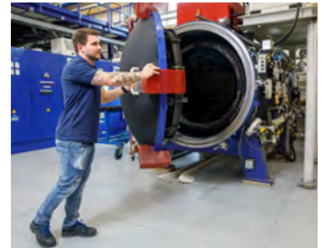
Filling a vacuum brazing furnace
